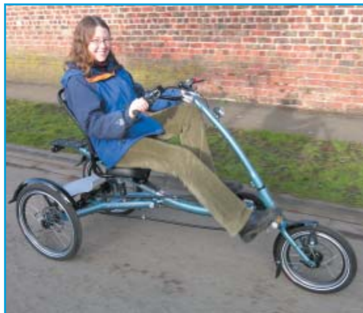
ABOVE: Handlebars adjust for reach and angle, so most riders should be able to achieve both knee clearance and comfort.
