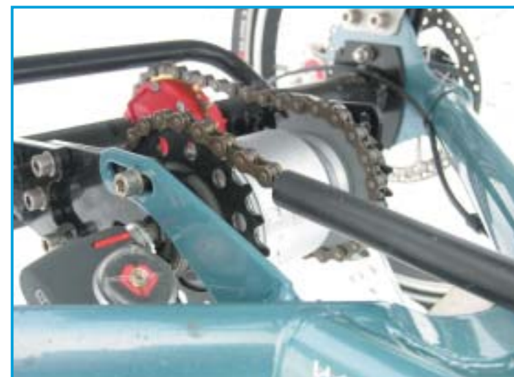
BELOW: Reverse gear comes via the coaster brake on the hub gear. This in turn drives the (red) differential unit on the rear axle, which splits the power evenly between the two rear wheels, even when, as you corner, the wheel on the outside has to go faster than the one on the inside of the bend.
