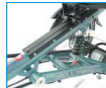
BELOW: The seat slides along the frame for leg-length adjustment, with plenty of travel for short and tall riders alike.
